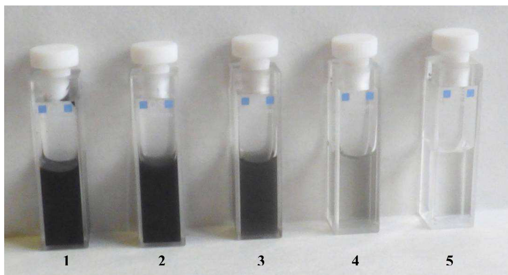
Figure 5. Digital photograph of as prepared 45 \text{mg mL}^{-1} graphene dispersion stabilized with FMNS (cuvette 1), the same dispersion diluted by a factor of 100 (2), 1000 (3), 5000 (4), and pure milli-Q water (5).
